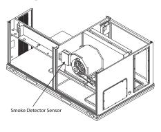
Fig. 18 - Typical Supply Air Smoke Detector Sensor Location
